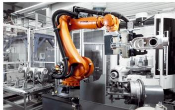
Robotic finishing work at a machine tool. The robot carries out machining jobs in addition to the automation task.
