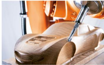
Free-form surface machining on a wooden model with the capability of processing extremely large CNC programs.
