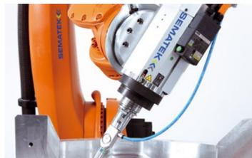
Machine hammer peening with a KR QUANTEC and KUKA.CNC.
